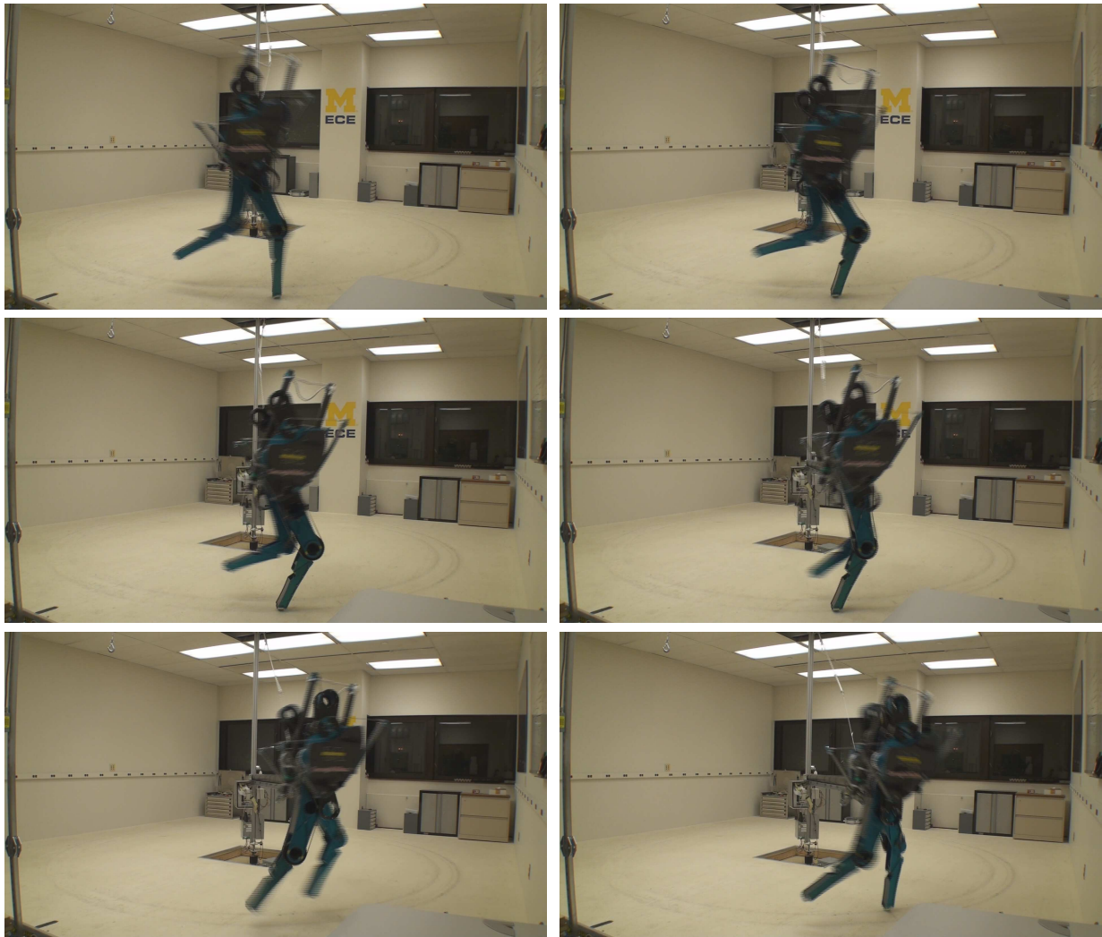
Fig. 8. A typical running step for MABEL. Snapshots are at an interval of 100 ms. A video of the running experiment is available on YouTube [22].
