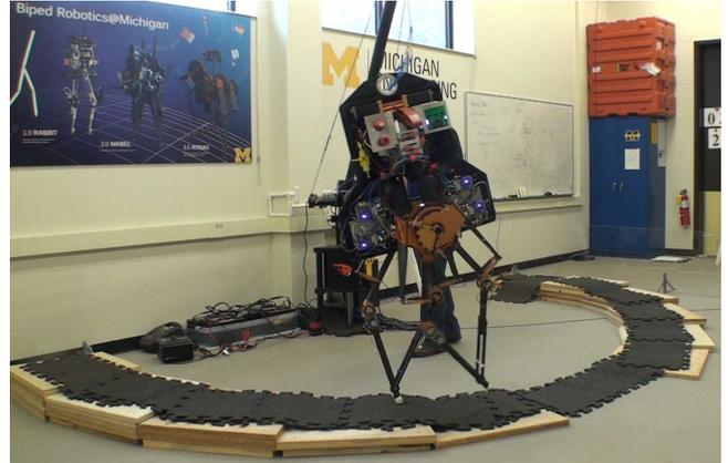
Fig. 1: MARLO, an ATRIAS 2.1 robot designed by the Dynamic Robotics Laboratory at Oregon State University, walks with unknown terrain heights.
