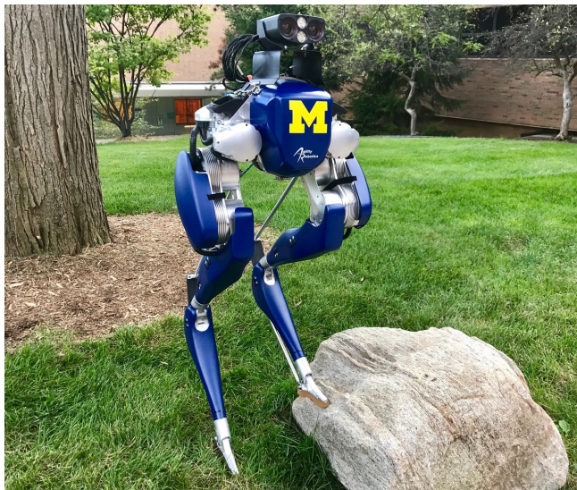
Fig. 1: Experiments were conducted on a Cassie-series robot designed by Agility Robotics. The biped robot has 20 degrees of freedom, 10 actuators, joint encoders, an IMU, and a Multisense S7 stereo camera.
