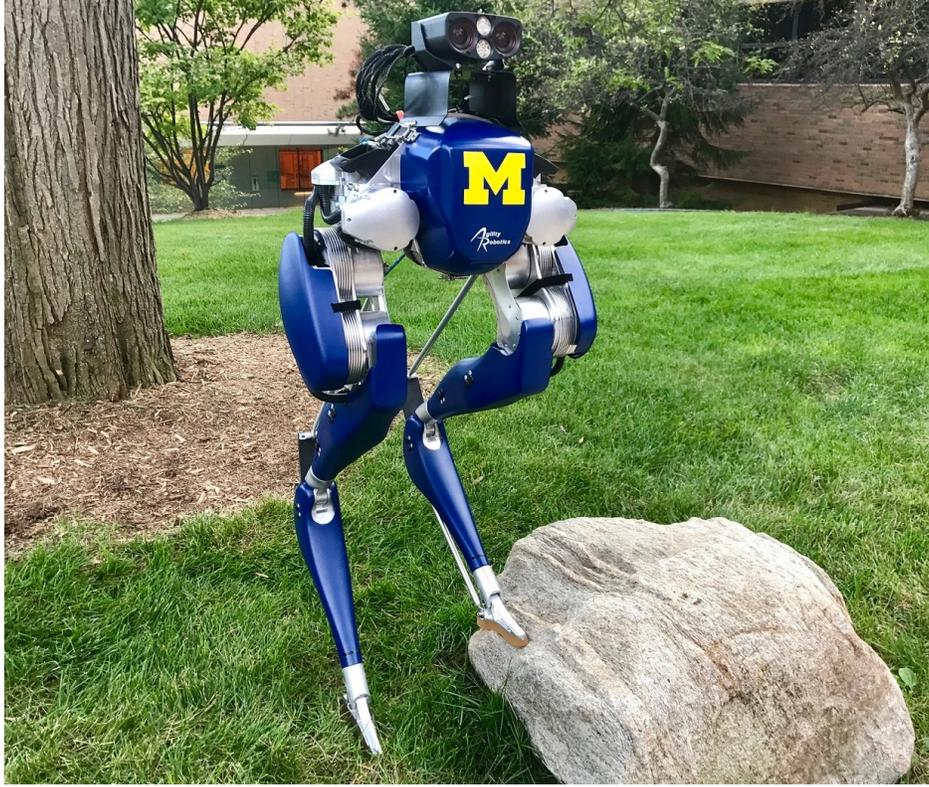
Figure 3.3: Cassie (Blue) is a biped robot developed by Agility Robotics. It has 20 degrees of freedom, 10 actuators and 4 springs. The robot is equipped with an inertial measurement unit, joint encoders. In this picture, a Multisense S7 stereo camera is also mounted.
