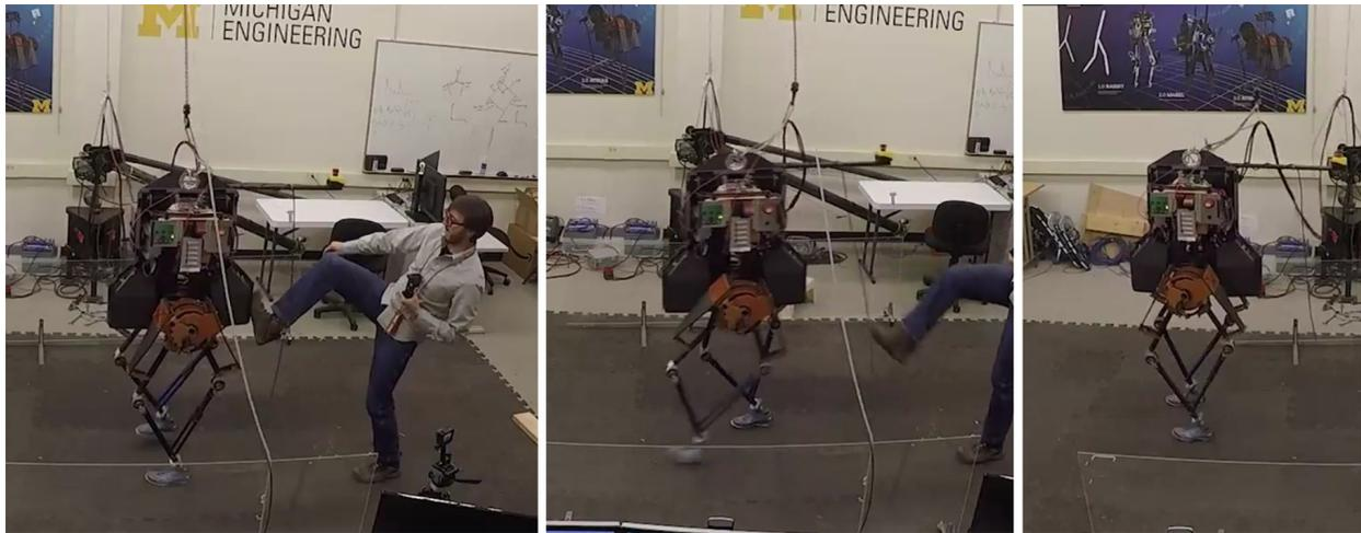
Figure 6.6: The posture adjustment function (PAF) (version 1) allows MARLO to withstand a large velocity disturbance of approximately 0.8 m/s.
