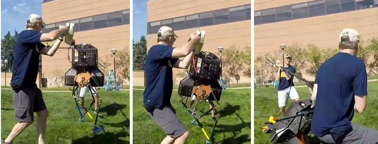
Figure 1.2: MARLO walking on the Wave Field. Without prior knowledge of the upcoming terrain, MARLO cannot adapt its gait to the large drop causing the robot to fall.
