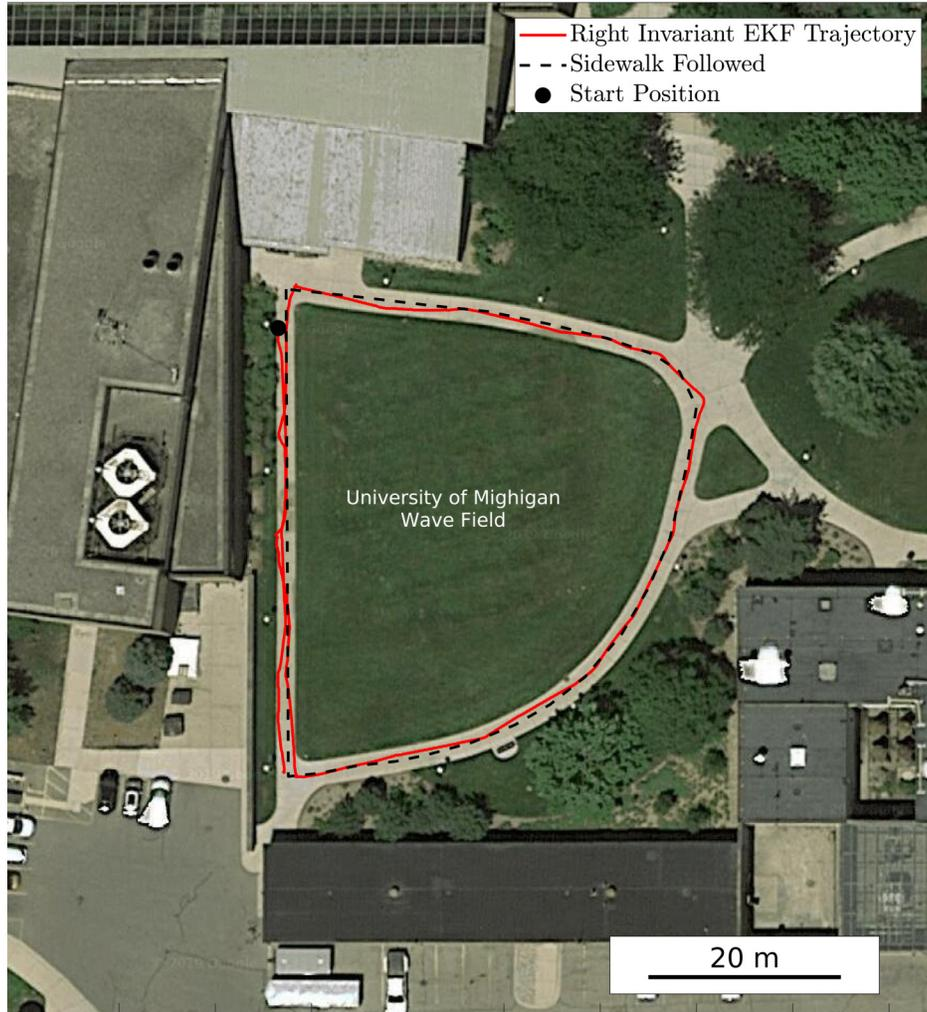
Figure 4.11: Long outdoor odometry experiment where Cassie walked roughly 200 m along a sidewalk over 7 minutes and 45 seconds.
