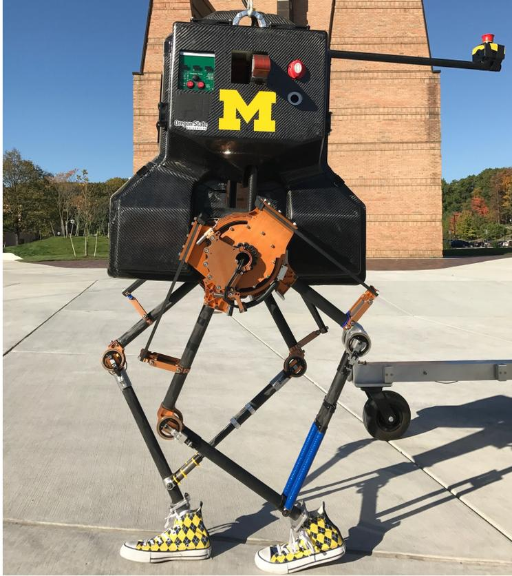
Figure 3.1: MARLO, the Michigan copy of an ATRIAS-series robot designed by the Dynamic Robotics Laboratory at Oregon State University
