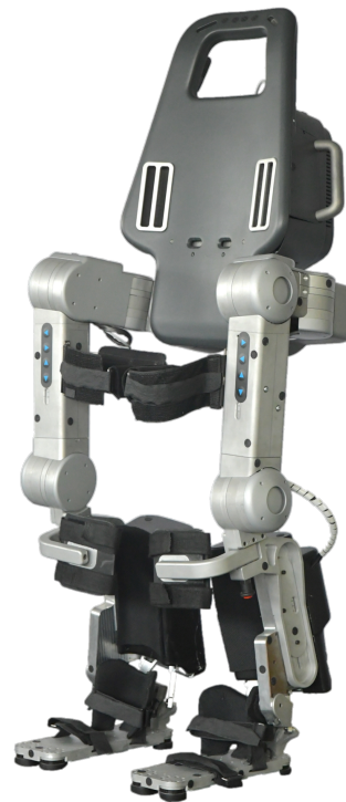
Fig. 1: ATALANTE: An exoskeleton designed by Wanderingcraft for people with paraplegia.
