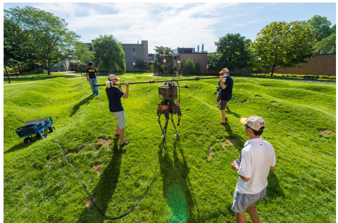
Fig. 1: Bipedal robot MARLO walked on the University of Michigan’s Wave Field, a sinusoidally varying grass terrain. Photo was taken by Roger Hart.
