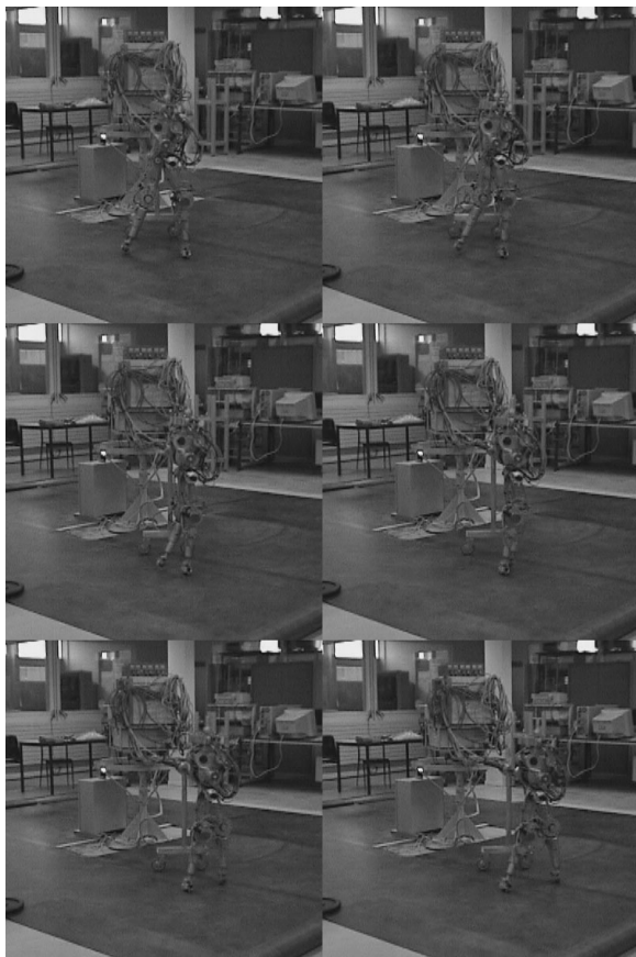
Fig. 11. Video frames of RABBIT taking a step. The interval between frames is 120 ms. Note the “training wheels” attached to the boom to provide a measure of safety.
