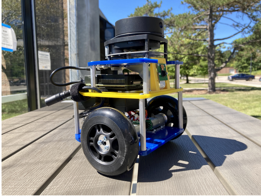
Figure 5.3: The same small mobile robot that we showed in Chapter 3.4.1. The user commands wheel speed. If both wheels move at the same speed, the robot moves in a straight line. If one wheel turns faster than the other, the robot turns toward the side of the slower wheel. Yet, somehow, our “Planning Team” has given us position trajectories (aka, position curves in \mathbb{R}^2 ), instead of velocity. We need to convert the position trajectories to velocity commands because our “Control Team” is still working on the position trajectory tracking controller for the robot. It will not be available until Chapter 10.
