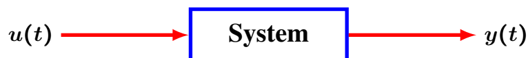
Figure 10.1: An Input-Output System. The signal u(t) represents the action of an actuator , such as a DC motor, a rocket engine, or a voltage supply. The output is a signal that is important to the system designer, such as the speed of a robot or the angle of a joint. If u(t) and y(t) are scalar-valued, then one has a Single-Input, Single-Output (SISO) System. If u(t) or y(t) are vectors, then one has a Multi-Input Multi-Output (MIMO) System.
