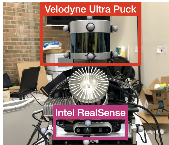
Figure 12.7: This figure shows the torso of Cassie Blue. We use it in practice to do our autonomy adventures!
