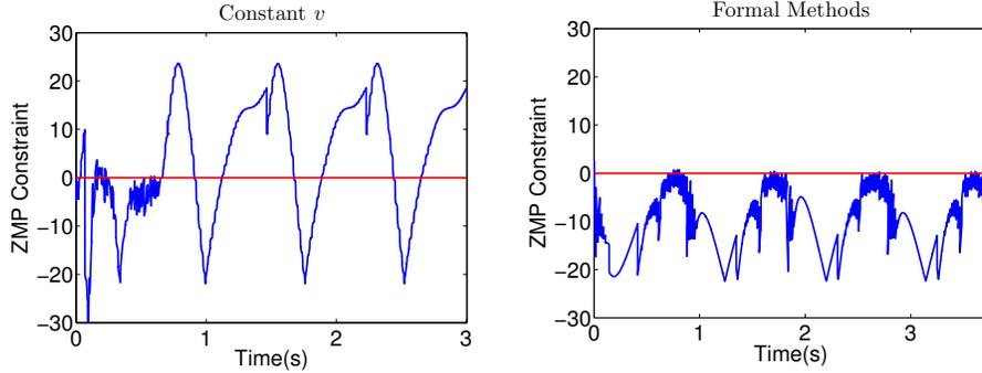
(a) Maximum violation of (C3) over four simulated steps. The upper bound of this constraint is equal to zero as illustrated by the horizontal red line. As we can see, the constant  $v$  controller causes this constraint to be significantly violated, while the formal methods controller obeys this bound.
