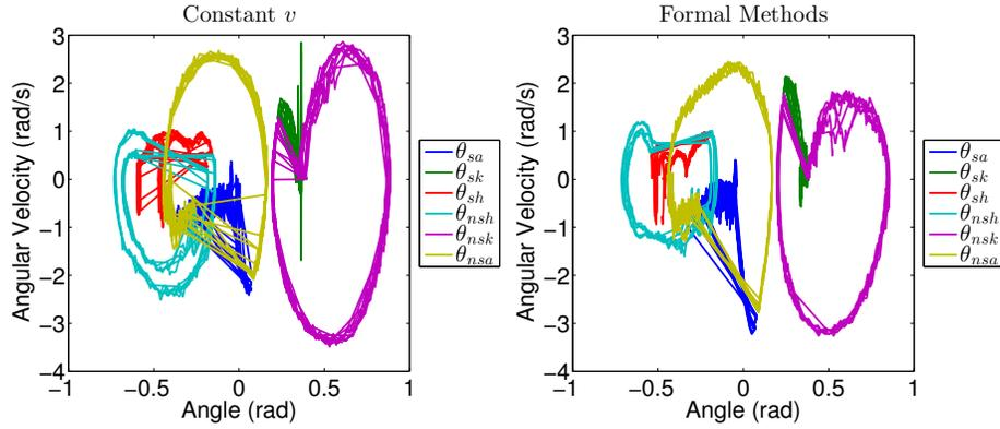
(a) Phase portrait for the state of the system  $(\theta, \dot{\theta})$ . The maximum allowed angular velocity,  $\pm 5 \text{ rad/s}$  (Constraint (C1)), was never violated by any joint in the robot under either controller.
