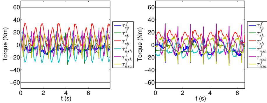
(b) The torques applied at each of the joints of the robots. The torque bounds of  $\pm 60 \text{ Nm}$  are illustrated with horizontal black lines (Constraint (C2)). The torque remains bounded under each of the controllers.
