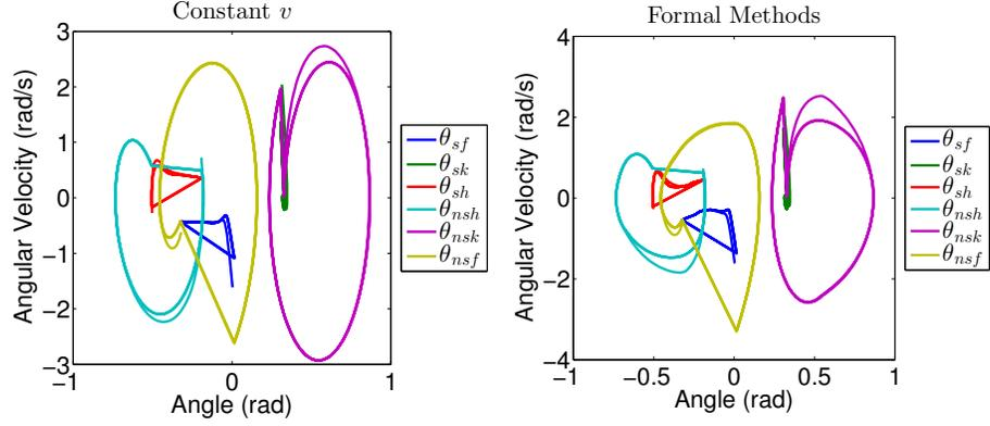
(a) Phase portrait for the state of the system  $(\theta, \dot{\theta})$  over four steps. The maximum angular velocity,  $\pm 5 \text{ rad/s}$  (Constraint (C1)), was never violated by the system under either controller.
