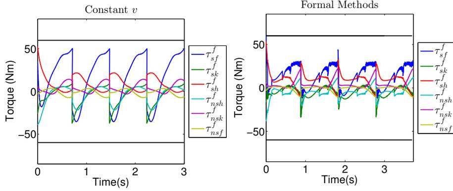
(b) The torques applied at each of the joints over four steps. The torque bounds of  $\pm 60 \text{ Nm}$  are illustrated with horizontal black lines (Constraint (C2)). The torque remains bounded under each of the controllers.
