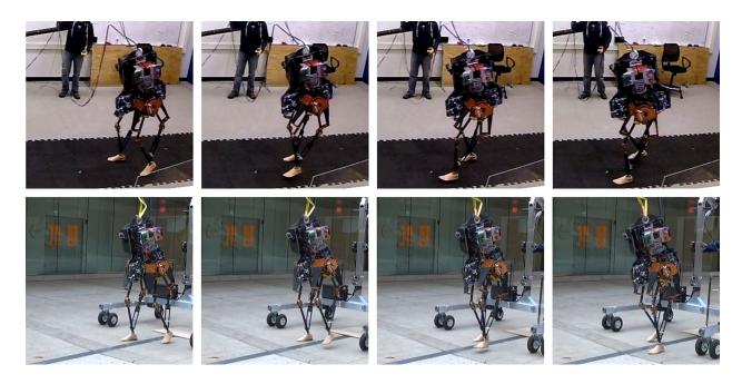
Fig. 6: Video snapshots from two 3D walking experiments. Frames are 200 ms apart. Videos of indoor (top row) and outdoor (bottom row) experiments are available online [28].
