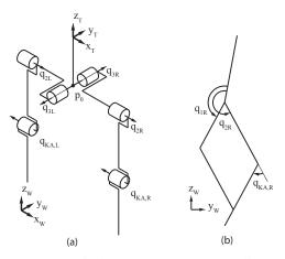
Fig. 2: Mechanical structure and coordinates for MARLO. (a) Conceptual diagram of rigid body model. (b) Each leg is physically realized by a four-bar linkage. The knee angle  $q_{KA,R}$  is related to the angles of the upper links as  $q_{KA,R} = q_{2R} - q_{1R}$ .
