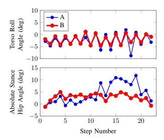
Fig. 5: Beginning-of-step torso and hip angles during two 3D walking experiments. In (A), a fixed torso offset was used. Adjusting the torso angle to control walking speed improved stability.
