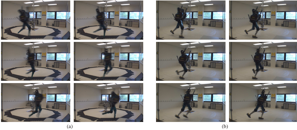
Fig. 18. Snapshots of a typical running step for (a) running with point-feet, and (b) running with passive feet, are shown at intervals of 100 ms. The snapshots progress temporally from left to right and from top to bottom.
