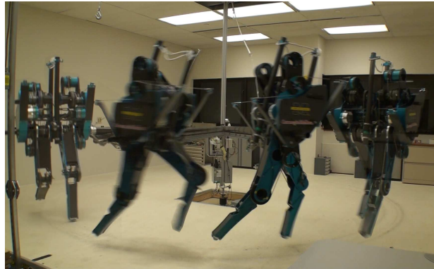
Fig. 1. A composite illustrating the dynamic and agile running gait obtained on MABEL.
