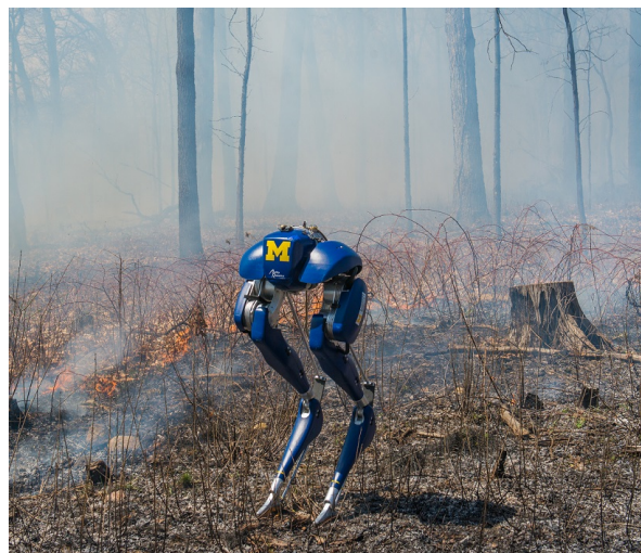
Fig. 1: Cassie Blue, one of Michigan’s Cassie-series robots designed by Agility Robotics. The robot is shown here participating in a controlled burn. It has 20 degrees of freedom, 10 actuators, joint encoders, and an IMU. The robot’s serial number is 001.
