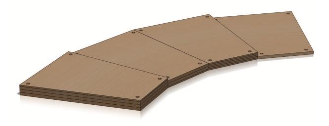
Figure 25: Plywood boards used to form a stair-stepped platform. By combining boards that are 1 inch (2.54 cm) and 0.5 inch (1.27 cm) thick, platforms of a desired height are assembled.
